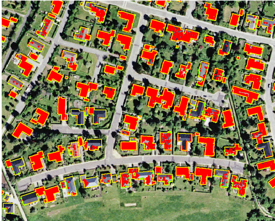
Figure 15. Laser scanning in built-up areas. The footprints are displayed inside buildings by red or green colour. Some of the buildings have none or only a few footprints because black roofs do not return the laser light. A DSM cannot be determined for such houses.
